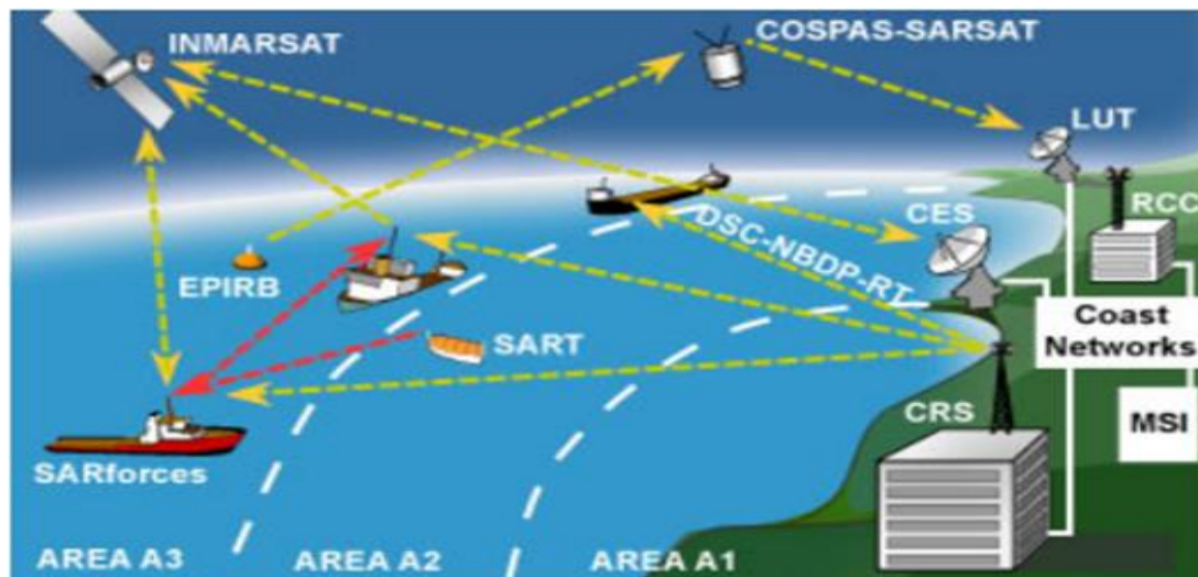
Figure 1. Functional requirements of the GDMSS System (Source: USCG-GMDSS-Guide-Booklet, 2019)
